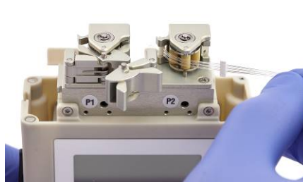
Figure 13: Inserting the OFM Tubing Set into the left fitting.
