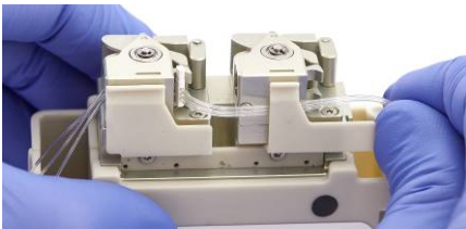
Figure 15: OFM Tubing Set is fixed with retaining springs in the pump.
