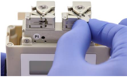
Figure 12: Opening of pump head using the snap mechanism.
